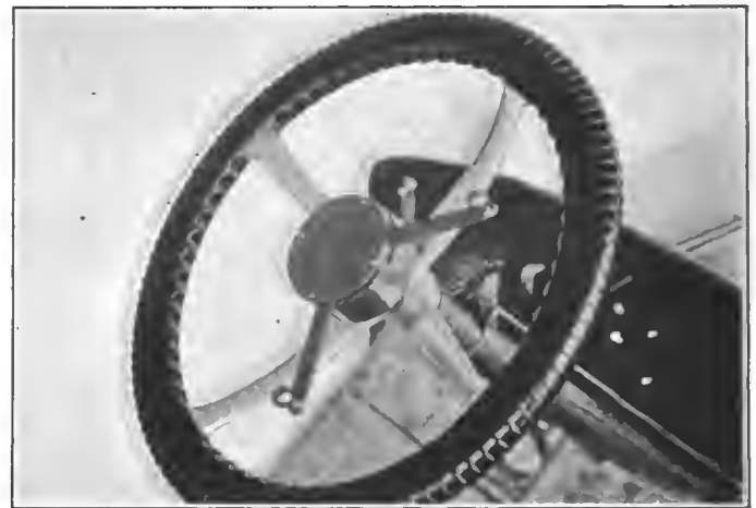
Lozier steering equipment, showing a large diameter fluted grip on the wheel, stout post, with secure anchorage at the foot-board
